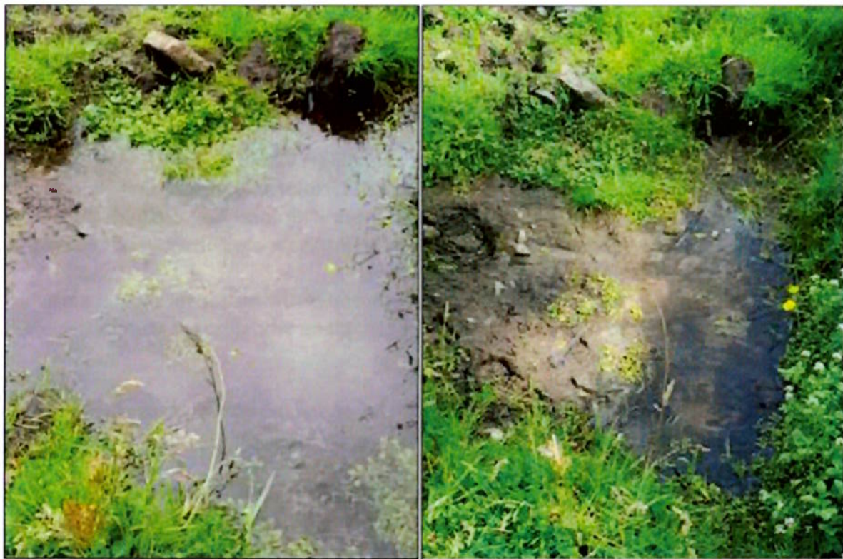
Figure 3.8. SP1 on the 11/07/22 i.e., pre-pumping (left) and after 10 days of pumping 22/07/22 (right). Note the very evident decrease in water levels.
